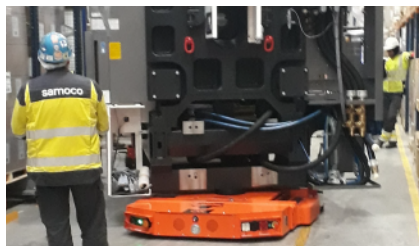
Manipulating equipment with the OX TBC-60 self propelled trolley at United Caps Hoboken
